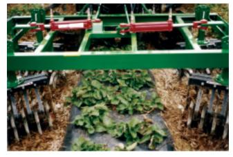
The cultivator frame consists of two channels which form the track for two sliding sub frames. The cultivating tools are mounted on the sub-frames and are hydraulically adjusted by the tractor operator. With this adjustment fine tuning of the cultivator to size of the crop size is done quickly when moving between different fields. This feature is especially useful for cultivating the edges of plastic mulch. The rolling cultivators move the soil laterally
