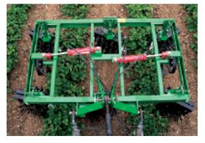
which will cover small weeds along the side of the plastic mulched bed or cover loose edges of plastic, but will not tear up the plastic if they come too close. A total of 16" of adjustment for each side of the row is possible by inter-changing the attachment points of the cylinders.
