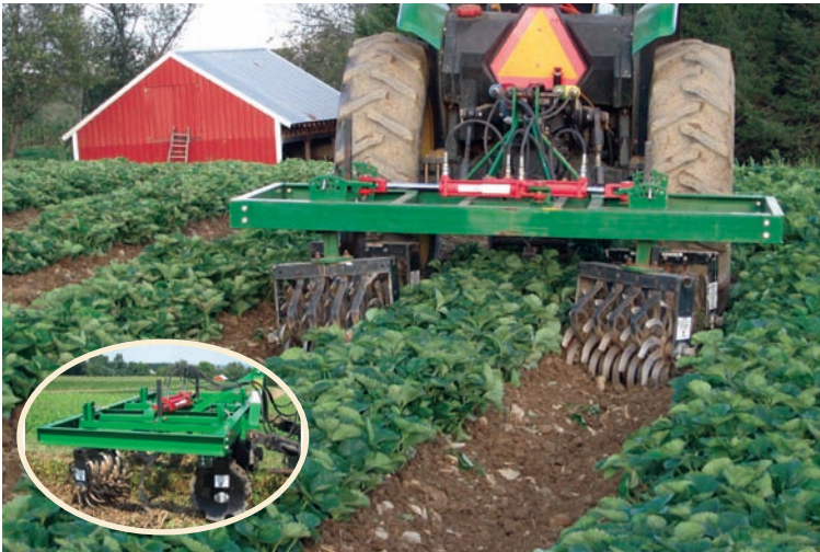
Hillside Cultivator Model CS is constructed with a strong frame and hydraulics for adjusting the distance between the cultivator gangs
