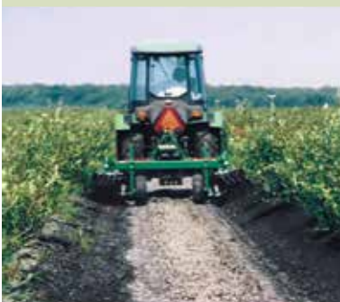
Hillside Cultivator Telescoping Frame for cultivating between blueberries or raspberries
