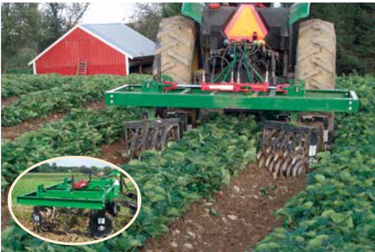
Hillside Cultivators are very effective for weed control between crop rows and renovating strawberries
