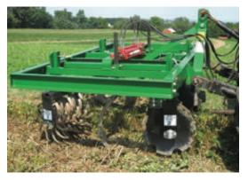
The **Eco Weeder** is a PTO driven machine with rotating vertical teeth that are manually moved between and around young plants. An attachment is available for straw removal in the spring.
