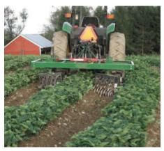
front position which are used to narrow the row and cut through the straw. A coil tine follows and fractures the soil which has been packed by foot traffic during harvest. The rolling cultivator in the rear rolls soil back toward the strawberry plants. Cultivating speed is 3-4 mph with two passes normal for each row. This machine is more economical and less disruptive of soil structure than a rototiller.
